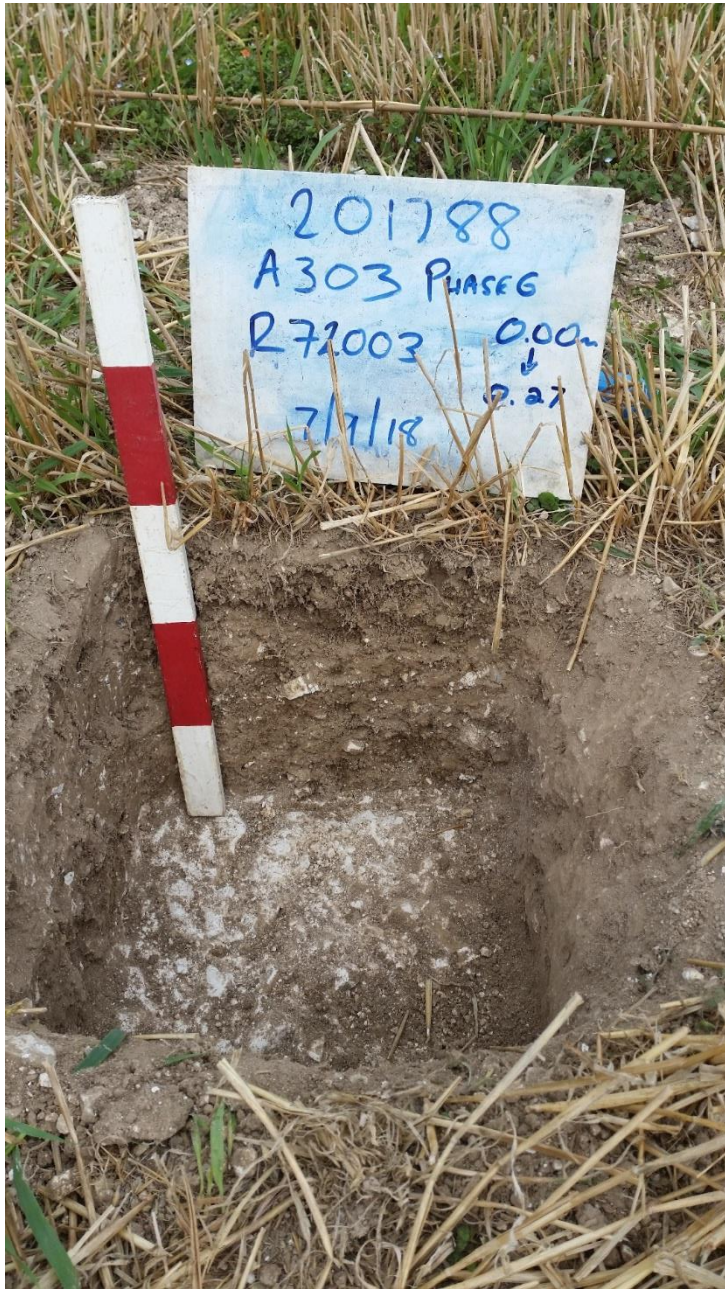
Plate 8-2. Inspection pit for borehole R72003
